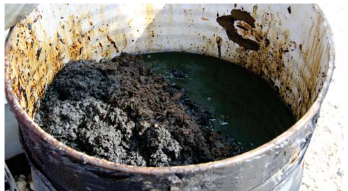
Sand, Wax and Solids Removed in Crude Oil Treater
